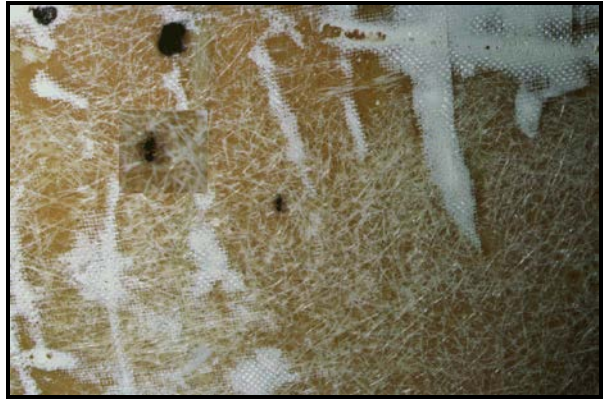
Fig 15. Preparation by gelcoat peeling alone.
