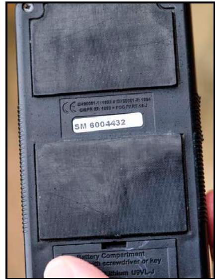
Worn electrodes like these will reduce sensitivity.
