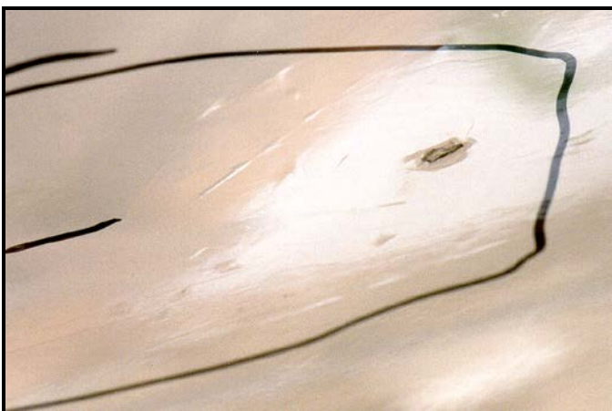
Fig 6: Fibre swelling in bare white gelcoat. Fibre swelling is not caused by osmosis, but by capillary action in fibre bundles behind the gelcoat.
