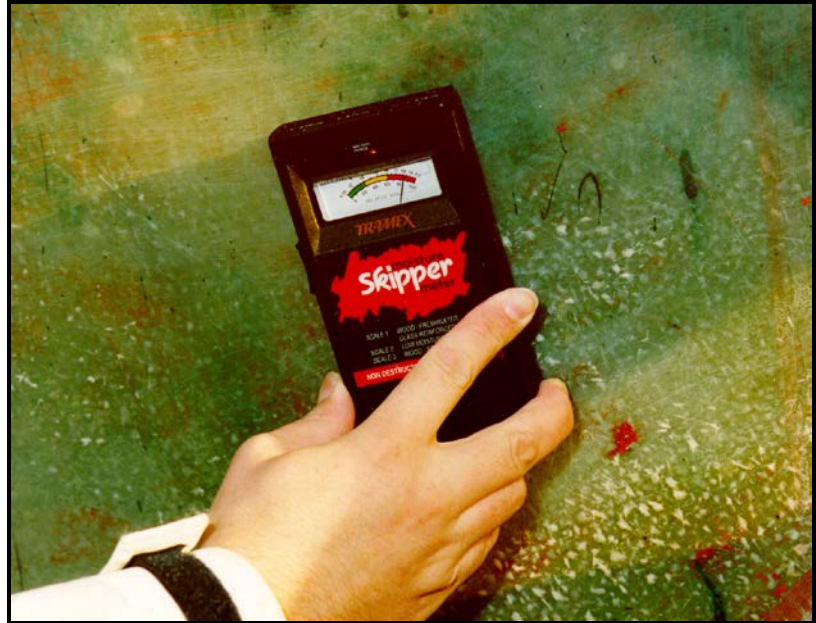
Fig 20. A Tramex Skipper meter being used on an exposed clear gelcoat. The white spots are caused by an effect known as 'fibre swelling', where bundles of glass reinforcement have absorbed moisture, which forces the filaments apart by capillary action. A pigmented gelcoat would only show small swellings at its surface.
