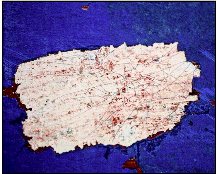
Fig 7: Antifouling coupon exposing gelcoat crazing.
