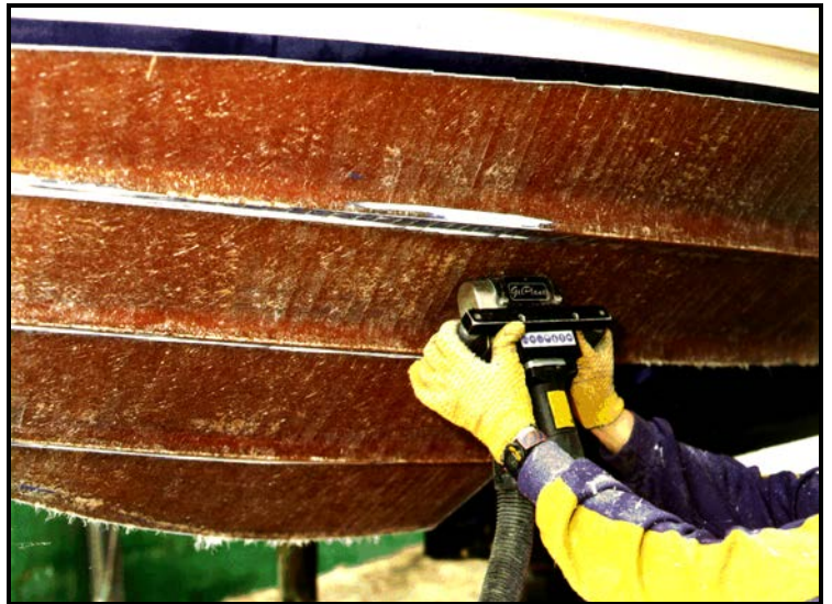
Fig 13. Gelcoat Peelers are ideal for bulk gelcoat removal, but note the very 'woolly' surface and unbound fibre left behind.
